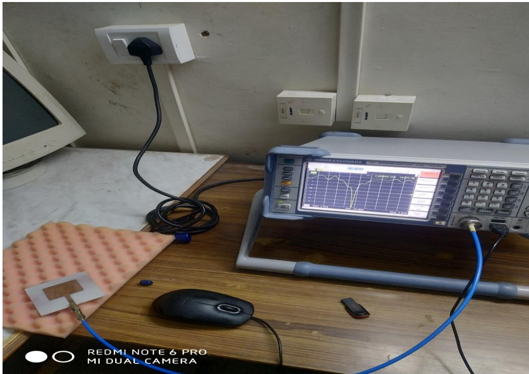
Figure 5.5 Testing antenna using R&S®ZVL Vector Network Analyzer
